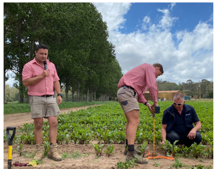
Elders agronomists Noel Jansz and Hugh McShane, along with Marc Intervera from Sentek Technologies, demonstrate the installation of a soil data monitoring probe.
